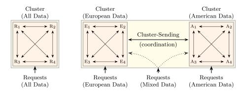
**Figure 1.** *Left*, a traditional fully-replicated resilient system in which all four replicas each hold all data. *Right*, a *sharded* design in which each resilient cluster of four replicas holds only a part of the data.
